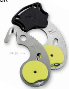
6H20DESIGNER: Benchmade BLADE STEEL: X15 T.N Stainless Steel (58-60HRC) BLADE OPENING: 0.50" (1.27cm) BLADE THICKNESS: 0.115" (2.92mm) WEIGHT: 2.30oz (65gm) HANDLE SPECS: 6H2O Steel w/ Yellow Kydex Overlay HARD SHEATH: Molded Delrin Snap-Fit (Varied Carry Options Available) HARD SHEATH WEIGHT: 0.36oz (10.21gm) OVERALL LENGTH: 4.25" (10.80cm) COUNTRY OF ORIGIN: USA BLADE CONFIGURATIONS: 6H20 (Includes Hard Sheath) \$53
