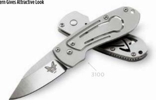
3100DESIGNERS: Bill McHenry & Jason Williams LOCKING MECHANISM: Auto-Levitator Lock BLADE STYLE & OPENER: Clip-Point, Auto-Levitator BLADE STEEL: 154CM Stainless Steel Hardened to 58-61HRC BLADE LENGTH: 1.95" (4.95cm) BLADE THICKNESS: 0.084" (2.13mm) OPEN: 4.75" (12.07cm) CLOSED: 2.84" (7.24cm) WEIGHT: 1.20oz (34gm) HANDLE SPECS: Stainless Steel HANDLE THICKNESS: 0.24" (0.61cm)
