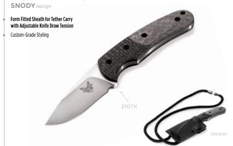
210DESIGNER: Mike Snody BLADE STYLE: Drop-Point Utility BLADE STEEL: S30V Premium Stainless Steel (58-60HRC) BLADE LENGTH: 2.125" (5.40cm) BLADE THICKNESS: 0.140" (3.56mm) WEIGHT: 2.50oz (70.87gm) HANDLE SPECS: Carbon Fiber Bolster w/ Silver G10 scales HANDLE THICKNESS: 0.392" (9.96mm) SHEATH: Kydex® Snap-Fit Tether Sheath **SHEATH WEIGHT:** 0.90oz (25.51gm) **OVERALL LENGTH:** 5.50" (13.97cm)
