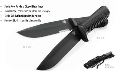
156DESIGNER: Benchmade BLADE STYLE: Combat/Survival Bowie BLADE STEEL: D2 Tool Steel (60-62HRC), BT Coated **BLADE LENGTH**: 6.10" (15.50cm) **BLADE THICKNESS**: 0.175" (4.45mm) **WEIGHT**: 9.60oz (272.16gm) **HANDLE SPECS**: Black Kraton® Overlaywith BILT® System **HANDLE THICKNESS**: 0.78" (1.97cm) **SHEATH**: Multi-Function Soft Sheath, Removable Pouch, Black Nylon SHEATH WEIGHT: 6.50oz (184.27gm) OVERALL LENGTH: 10.90" (27.69cm) **COUNTRY OF ORIGIN: USA**
