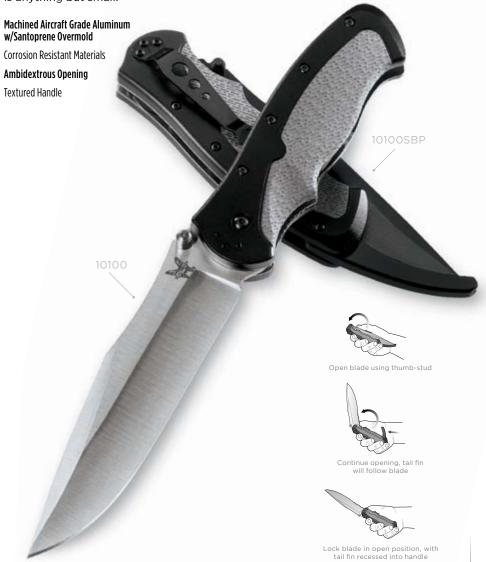
10100 DESIGNER: Benchmade LOCKING MECHANISM: Locking-Liner BLADE STYLE: Clip-Point BLADE STEEL: 440C Stainless Steel (58-60HRC) BLADE LENGTH: 5.20" (13.21cm) BLADE THICKNESS: 0.118" (2.98mm) OPEN: 10.25" (26.06cm) CLOSED: 6.70" (17.02cm) WEIGHT: 6.70oz (189.94gm) **HANDLE SPECS:** Machined 6061-T6 Aluminum with Santoprene Overmold **HANDLE THICKNESS:** 0.76 " (19.33mm) **COUNTRY OF ORIGIN:** Taiwan **BLADE CONFIGURATIONS: 10110 \$100, 10110SBP \$110**
