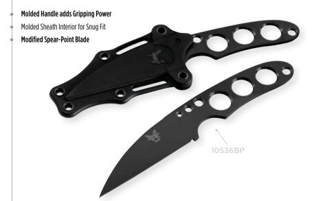
10536DESIGNER: Mike Snody BLADE STYLE: Modified Wharncliff BLADE STEEL: AUS-8 Stainless Steel (58-60HRC), BP Coated BLADE LENGTH: 3.28" (8.33cm) BLADE THICKNESS: 0.123" (3.12mm) WEIGHT: 2.30oz (65.2gm) HANDLE SPECS: AUS 8 Stainless Steel, Skeletonized, Full Tang HANDLE THICKNESS: 0.123" (3.12mm) SHEATH: Snap-Fit Molded Kydex®/ Thermoplastic With Tether OVERALL LENGTH: 7.38" (18.79cm) COUNTRY OF ORIGIN: Taiwan **BLADE CONFIGURATIONS: 10536BP** \$50
