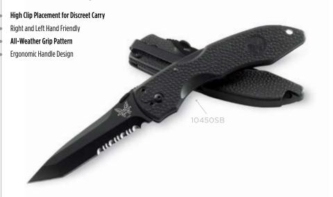
10450 DESIGNER: Benchmade LOCKING MECHANISM: Lock Back BLADE STYLE & OPENER: Modified Tanto; Ambidextrous Thumb-Disk BLADE STEEL: N690 Stainless Steel (58-60HRC) BLADE LENGTH: 3.50" (8.89cm) BLADE THICKNESS: 0.115" (2.92mm) OPEN: 8.30" (21.08cm) CLOSED: 4.80" (12.18cm) WEIGHT: 2.88oz (81.65gm) HANDLE SPECS: Molded Thermoplastic; Movable Steel Carry-Clip HANDLE THICKNESS: 0.45" (1.15cm) COUNTRY OF ORIGIN: Taiwan **BLADE CONFIGURATIONS: 10450SB \$45**
