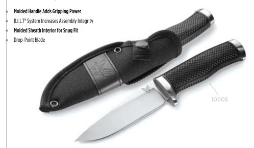
10505DESIGNER: Mel Pardue BLADE STYLE: Drop-Point BLADE STEEL: 440C Stainless Steel (58-60HRC) BLADE LENGTH: 4.48" (11.38cm) BLADE THICKNESS: 0.139" (3.53mm) WEIGHT: 6.40oz (181.44gm) HANDLE SPECS: Polypropylene w/ Black Kraton® Overmold; w/ BILT® System HANDLE THICKNESS: 0.88" (2.23cm) SHEATH: Black Ballistics Nylon w/ Belt Loop OVERALL LENGTH: 9.11" (23.14cm) COUNTRY OF ORIGIN: Taiwan BLADE CONFIGURATIONS: 10505 \$65
