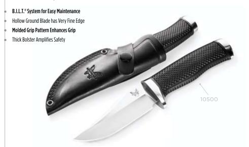
10500DESIGNER: Mel Pardue BLADE STYLE: Clip-Point Bowie BLADE STEEL: 440C Stainless Steel (58-60HRC) BLADE LENGTH: 3.95" (10.03cm) BLADE THICKNESS: 0.139" (3.53mm) WEIGHT: 6.16oz (174.633gm) HANDLE SPECS: Polypropylene w/ Black Kraton® Overmold; w/ BILT® System HANDLE THICKNESS: 0.88" (2.23cm) SHEATH: Black Leather w/ Belt-Loop OVERALL LENGTH: 8.58" (21.79cm) COUNTRY OF ORIGIN: Taiwan BLADE CONFIGURATIONS: 10500 \$65
