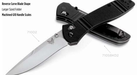
710 DESIGNER: Bill McHenry & Jason Williams LOCKING MECHANISM: AXIS Lock BLADE STYLE & OPENER: Modified Clip-Point; Dual Thumb Stud BLADE STEEL: D2 Tool Steel (60-62HRC) BLADE LENGTH: 3.98" (10.11cm) BLADE THICKNESS: 0.115" (2.92mm) OPEN: 8.80" (22.34cm) CLOSED: 4.98" (12.65cm) WEIGHT: 4.68oz (132.68gm) HANDLE SPECS: Black G10 Scales, Double 410 Stainless Steel Liners; Movable Steel Carry-Clip HANDLE THICKNESS: 0.48" (1.22cm) COUNTRY OF ORIGIN: USA e) AXIS
