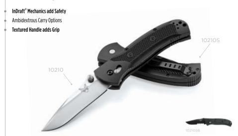
10210DESIGNER: Mel Pardue LOCKING MECHANISM: Rolling Lock® BLADE STYLE & OPENER: Drop-Point Utility; Ambidextrous Thumb-Studs BLADE STEEL: AUS-8 Stainless Steel (58-60HRC)
