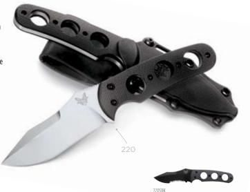
220 DESIGNER: Mike Snody BLADE STYLE: Gotham Swedged Clip-Point BLADE STEEL: 154CM Stainless Steel (58-61HRC) BLADE STYLE: Gottam Swedged Clip-Point BLADE STEEL: 154 Stainless Steel (58-61HRC) BLADE LENGTH: 3.40" (8.64cm) BLADE THICKNESS: 0.160" (4.06mm) WEIGHT: 4.56oz (129.27gm) HANDLE SPECS: Full-Tang; Skeletonized G10 Scales HANDLE THICKNESS: 0.51" (12.95mm) SHEATH: Molded Kydex® w/Belt Loop OVERALL LENGTH: 7.45" (18.92cm) COUNTRY OF ORIGIN: USA
